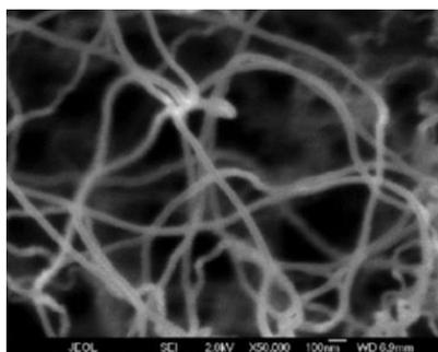
Figure 1 – Z.F. Ren, carbon nanotubes shown under electron microscope, 1998. (© Nano-Lab, Inc.)<sup>5</sup>
