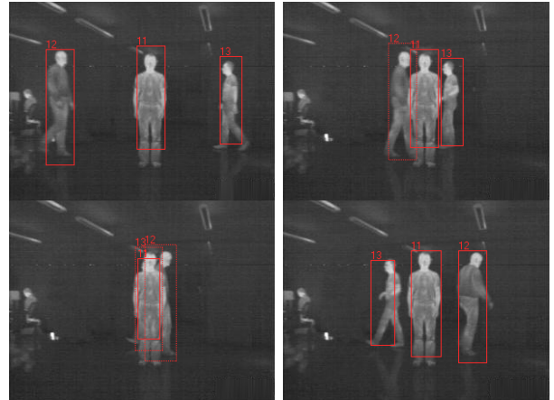
Fig. 5. Selected thermal images from the sequence showing the output from the tracker before, during and after the occlusion of three simultaneously tracked persons. The bounding boxes corresponding to occluded persons are marked by a dotted line.
