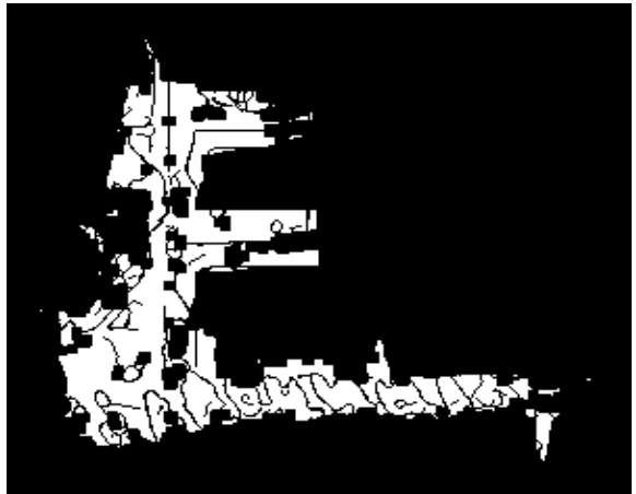
Fig. 8. The combined binary image of free points (reduced using morphological erosion with a square structuring element of size 5 \times 5 pixels) and edges in I_e .
