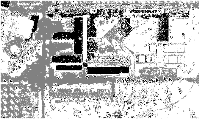
(a) Ground (gray) and building (black) estimates. The white cells are unexplored or unknown.
