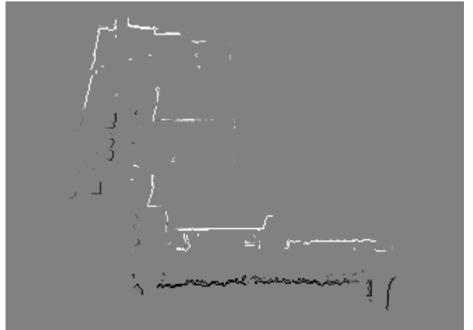
Fig. 2. An example of a probabilistic semantic map created with the approach described in the text. White cells denote high probability of walls and dark cells show outlines of non-building entities.
