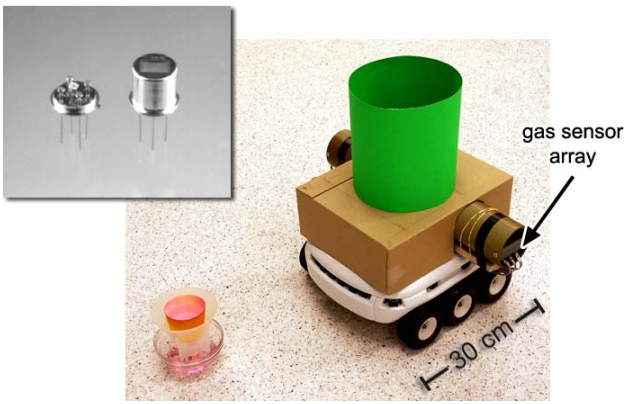
Fig. 1. Koala robot with the Örebro Mark III mobile nose and the gas source used in the experiments. The small image in the top left corner shows a Figaro gas sensor used in the Mark III mobile nose.
