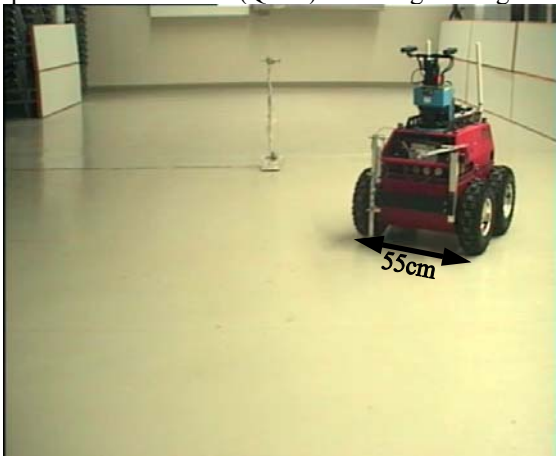
Figure 1: The robot Arthur, equipped with the gas sensor system. The main unit is inside the robot. Two sensors are mounted on the stiff extension on the front, four sensors are mounted at the vertical rod on the right side, the last two sensors are situated at the back end edges. In the middle of the room, the first version of the automatic source is shown.
