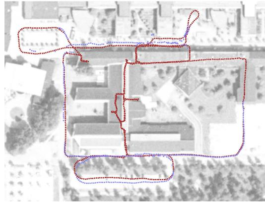
Fig. 6. DGPS data  $x^{DGPS}$  (blue) with aligned SLAM estimates  $\hat{x}$  (red) displayed on an aerial image. The squares show the SLAM and DGPS poses for which the number of satellites used to obtain the DGPS measurement was considered acceptable.
