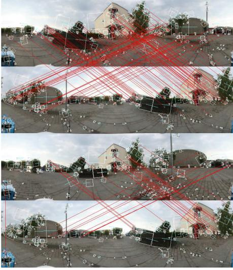
Fig. 2. Example of loop closing detection outdoors. The distance to the extracted features is comparably large. The top figure shows feature matches at a peak of the similarity value  $S_{678,758} = 0.728$ , whereas the lower figure shows the matches two steps away  $S_{680,758} = 0.286$  ( $\sim 3$  meters distance). The pose variance  $\sigma_{x_v}^2$  and  $\sigma_{y_v}^2$  was estimated to be  $2.16 \text{ m}^2$ .
