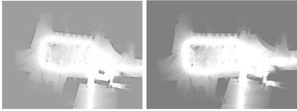
Fig. 9. Visualized map using laser range data to compare the accuracy of using (left) the estimated covariance for each poses and (right) using a constant covariance, where the constant covariance is the mean of the estimated covariances.
