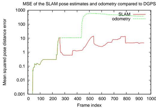
Fig. 10. The MSE of the Euclidean distance between the ground truth position obtained from DGPS readings  $x^{DGPS}$  and the SLAM estimate of the robot pose  $\hat{x}$  for different states of the maps as frames are added. Drops in the MSE indicate that the consistency of the map has been increased.
