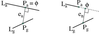
Fig. 5. The line  $L_g$  with its midpoint  $P_g = (x_m, y_m)$ , the line  $L_a^i$ , and the normal to  $L_a^i$ ,  $e_n$ . To the left,  $P_g = \phi$  since  $\phi$  is on  $L_a^i$  and to the right,  $P_g$  is the endpoint of  $L_a^i$  since  $\phi$  is not on  $L_a^i$ .
