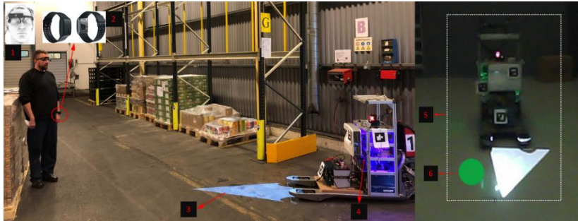
Figure 1. (1) Eye-tracker worn by a participant (2) Empatica E4 band used for measuring electrodermal activity. (3) SAR projection “Arrow” projected on the shared floor space to convey robot’s navigation intent. (4) Robot (a retrofitted Automatic guided vehicle - AGV) with SAR intention communication system. (5) The defined area of interest AOI-Robot. (6) Eye gaze fixation.
