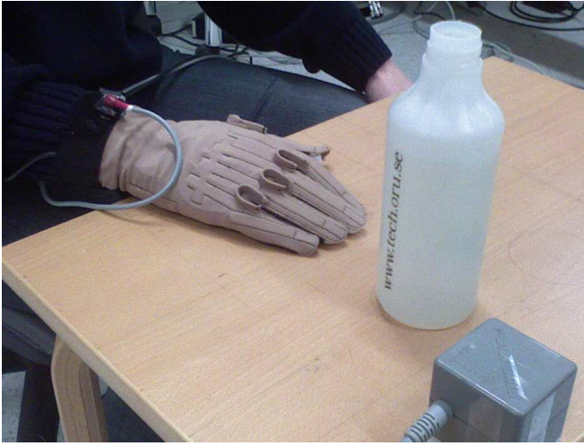
Fig. 6. The experimental setup with the data glove and the 6D tracker used for data collection.
