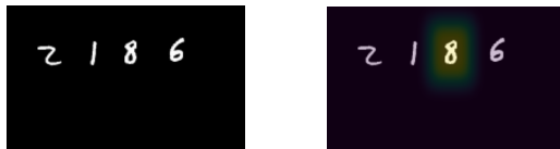
Figure 2: On the left, an example of a handwritten year. On the right, the attention map for the digit ‘8’ as a generalised normal distribution. Intuitively, we can view generalised normal distributions as differentiable bounding boxes. This allows gradients to flow from a downstream classification network to the regression component.
