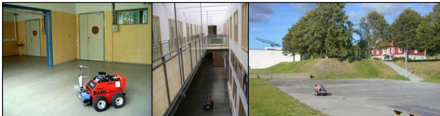
Fig. 2. The prototype pollution monitoring robot during the mission in the experimental environments: an enclosed indoor area (left), a part of a long corridor with open ends and a high ceiling (center), and an outdoor scenario (right).
