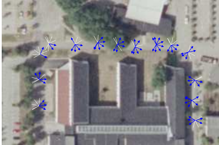
Fig. 5. Classification of images used as a virtual sensor pointing at the two classes (blue arrows indicate buildings and white lines non-buildings).
