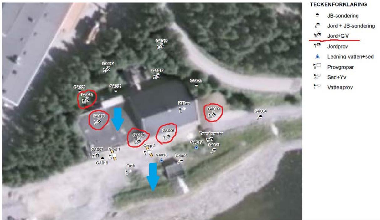
**Figure 3.** Sampling plan from Iggesund hard chromium plating site with the sampling points indicated by red circles. The waters flow direction is shown with blue arrows.
